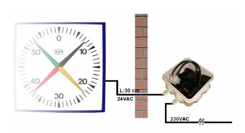
If the clock is run by edge of pool, you will also provide a lengthening of the cable connecting stopwatch to the transformer.
